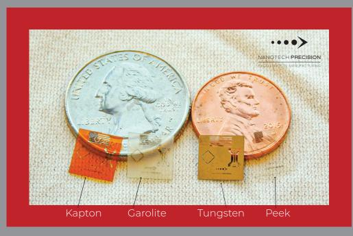
As the demand continues to grow to produce everything smaller and smaller, organizations within the precision manufacturing industry must continually adapt to stay relevant. Nanotech Precision is yet again showcasing its ability to do that, this time utilizing the stability and versatility of its Femto Laser System to machine one design in four different materials.
